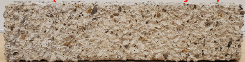
All Bloc™ - Post Freeze Thaw (Zero failure at 323 cycles)
