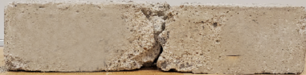
Control - Post Freeze Thaw (Failure at 59 cycles average)
